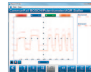
Target-actual comparison – by means of automatic measurement configuration and existing reference curves
