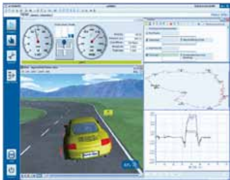
The screenshot shows PUMA Open including a 3D online animation of maneuver and track, a graphical testrun sequence and a recorder for data acquisition
