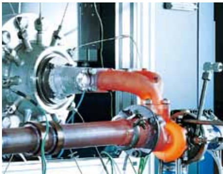
AVL turbocharger testbed and turbocharger during hot gas test.
