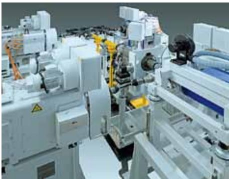
AVL testbeds with prime mover as IC engine substitute for front-wheel drive vehicles with transversely mounted engine.
