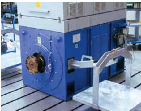
Highly precise, pendulum mounted, robust AC drive system with a state-of-the-art 4Q-IGBT converter for speed and torque controlled operation. A real-time torque calculator also provides the shaft torque of the machine in addition to the electric torque (air-gap torque).
