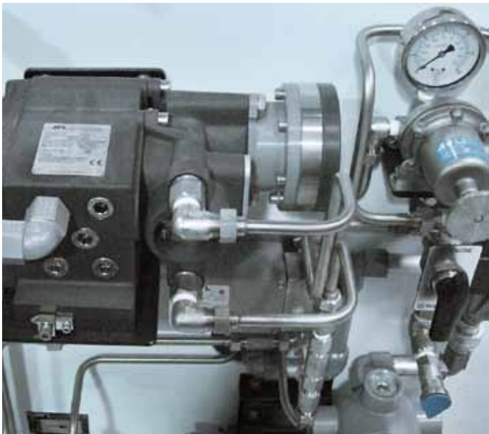
AVL PLU131 Flow Meter in a component test rig.
