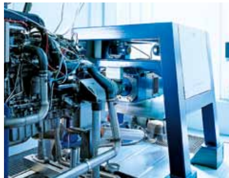
Highly dynamic, compact AC drive system for testing combustion engines consisting of state-of-the-art permanent magnet motor and IGBT frequency converter for 4Q operation with a digital real-time interface. Enables, together with a portal frame, testing of the original exhaust system.
