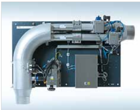
The CVS valve matrix is integrated into the AMA i60 COMBI cabinet. The compact dilution unit is prepared for wall or ceiling mounting to perfectly fit the testbed conditions.
