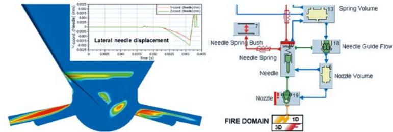
Coupling of AVL BOOST™ HYDSIM and AVL FIRE™ allowing for prediction of lateral needle forces and displacements
