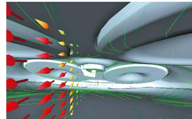
Flow pattern in a gasoline engine
