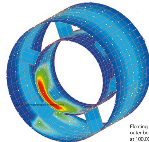
Floating bushing – inner and outer bearing oil film pressure at 100,000 rpm
