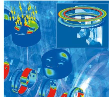
Four cylinder inline engine – friction in lubricated crank-train contacts
