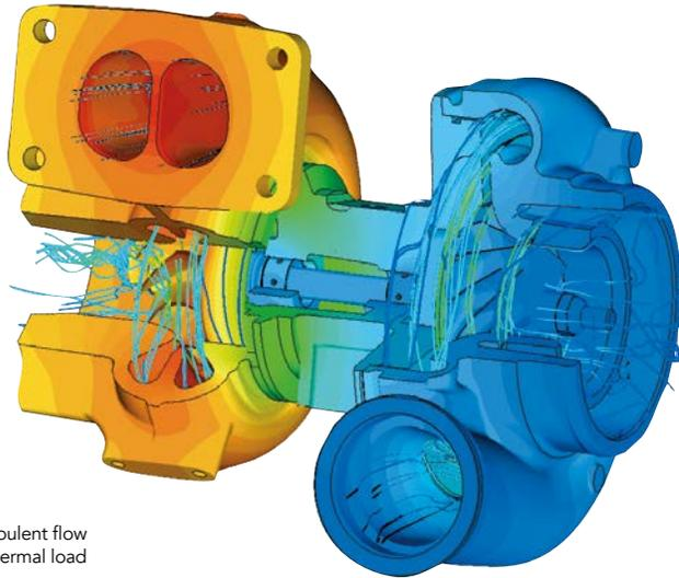
Complex turbulent flow and thermal load
