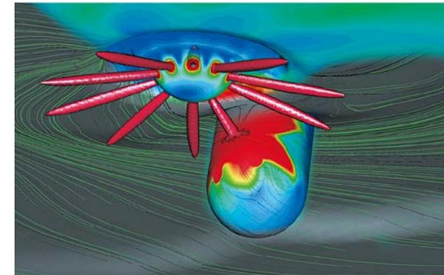
Gas injection onto a glow plug
