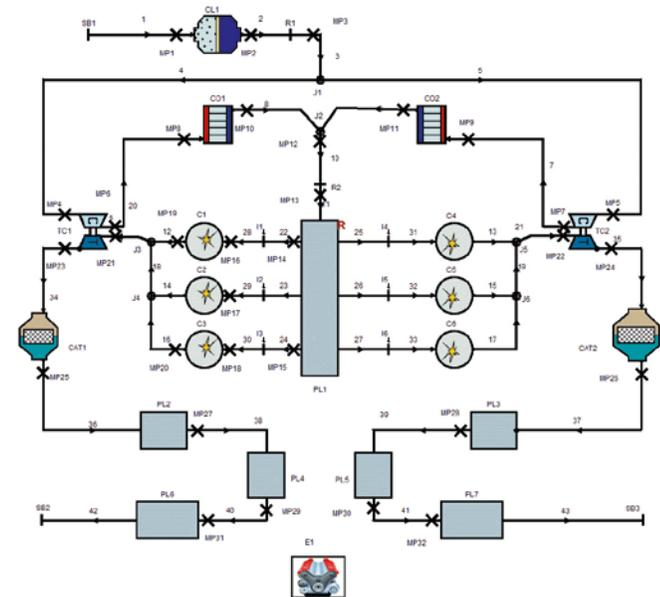
AVL BOOST™ model: 6 cylinder bi-turbo Ottomotor
