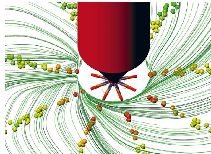
Cavitating internal nozzle flow applied as input for combusting in-cylinder flow
