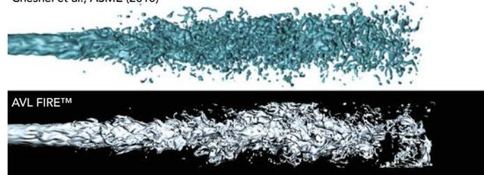
Application of LES together with the Volume-of-Fluid surface tracking method to capture spray propagation details
