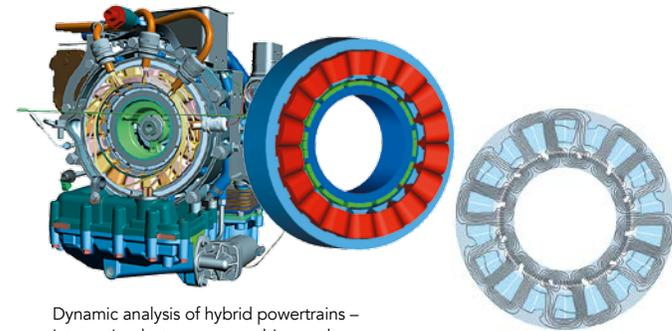
Dynamic analysis of hybrid powertrains – interaction between e-machine and IC engine (AVL EXCITE™)
