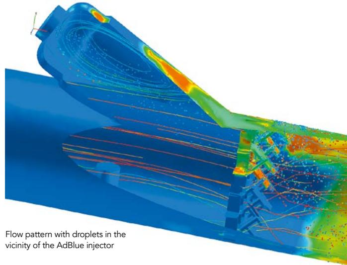
Flow pattern with droplets in the vicinity of the AdBlue injector
