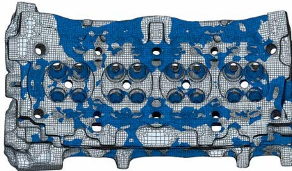
Von Mises stresses during quenching simulated by AVL FIRE™; five seconds after submerging
