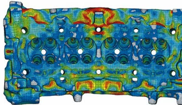
Von Mises stresses during quenching simulated by AVL FIRE™; 30 seconds after submerging
