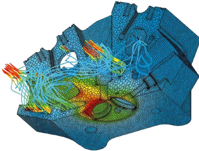
Coolant flow through the thermally loaded cylinder head
