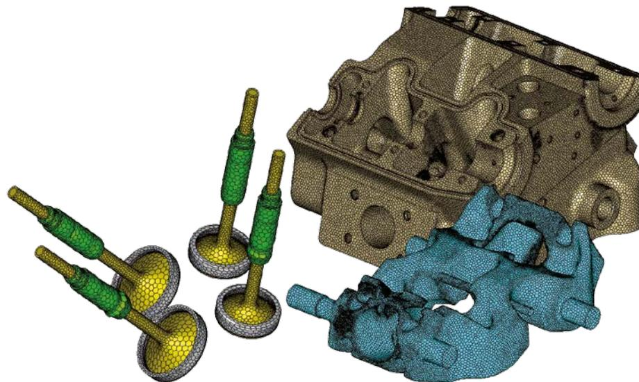
Multiple domains discretized in a single meshing step
