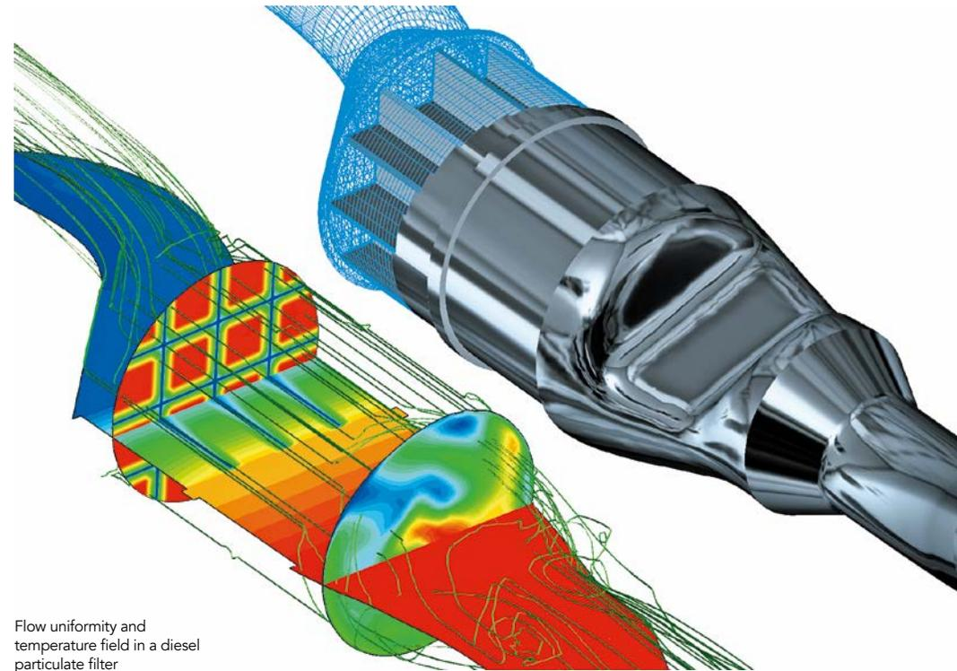
Flow uniformity and temperature field in a diesel particulate filter
