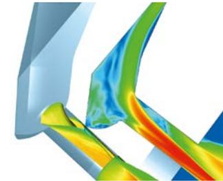
LES applied on a realistic diesel injector featuring three-phase flow and needle movement
