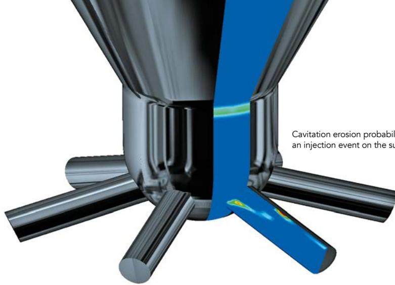
Cavitation erosion probability averaged over an injection event on the surface of the spray hole
