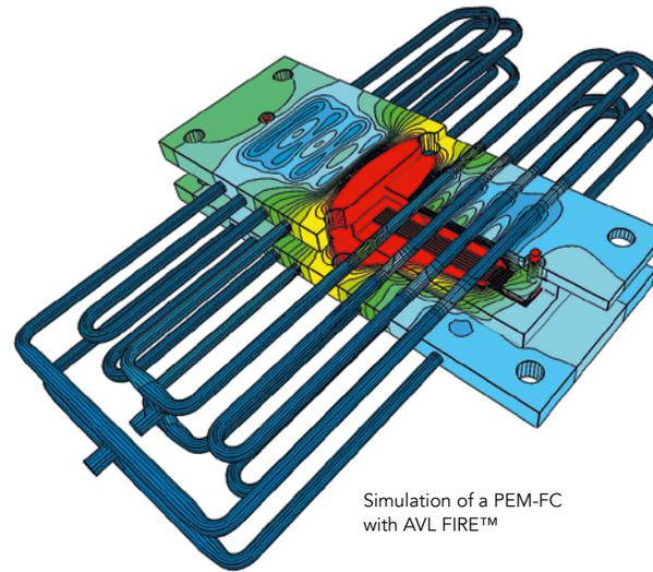
Simulation of a PEM-FC with AVL FIRE™
